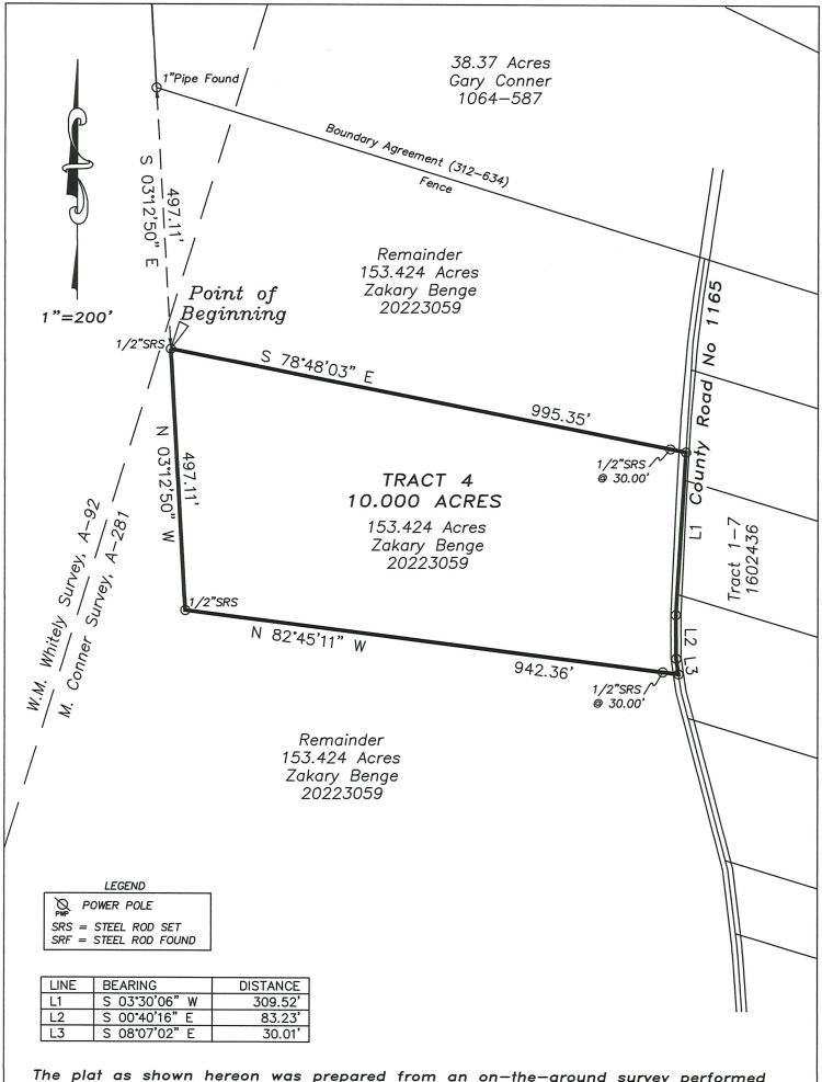
The plat as shown hereon was prepared from an on—the—ground survey performed under my supervision during the month of August, 2022.
