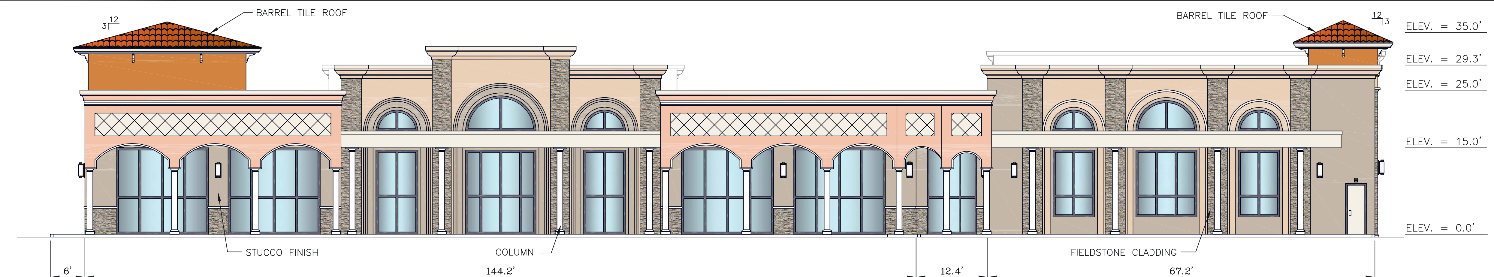
BUILDING II - SOUTH (FRONT) ELEVATION 1 INCH = 10 FEET
